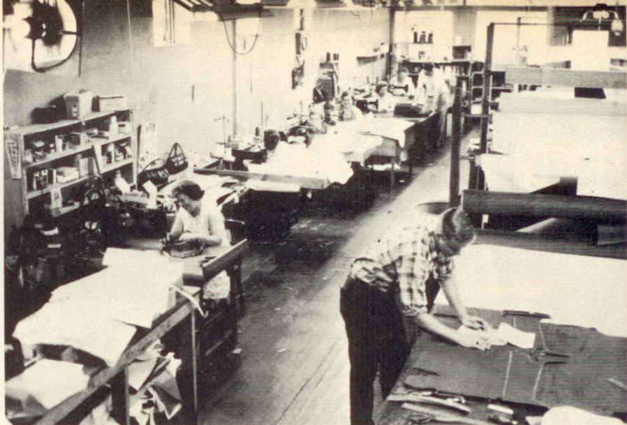
Assembly line production of tailor-made interior components. Several interior shops specialize in such work, allowing the aircraft owner to install it himself and save the cost of a custom job
